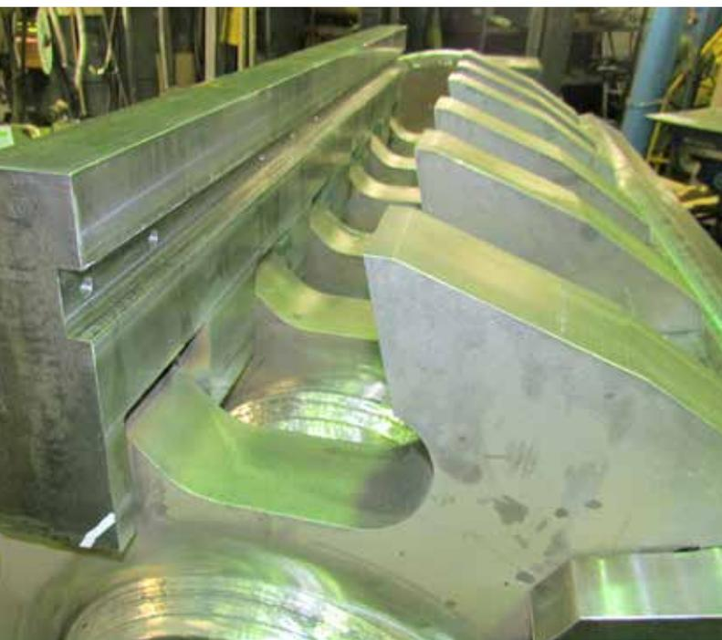
Detail of Prise™ 3 rotor with hammers
